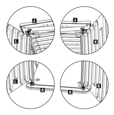
From inside the shed, install four **Screws (AA)** into the roof, two on each side wall.
